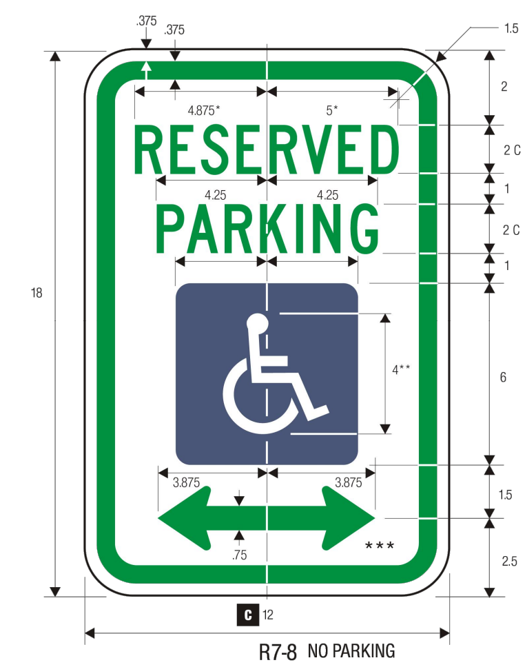
R7-8 NO PARKING LEGEND - GREEN (RETROREFL), WHITE SYMBOL ON BLUE (RETROREFL) BACKGROUND - WHITE (RETROREFL)
